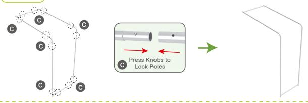
**STEP 03** Connect support poles onto frame.
