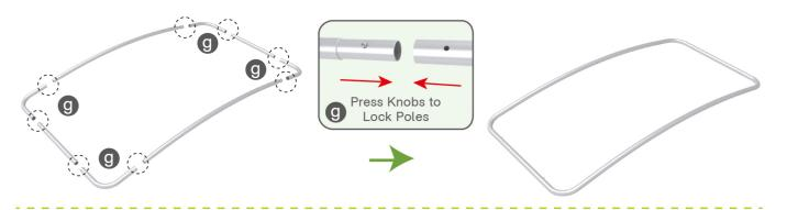
STEP 03 Connect support poles onto frame.
