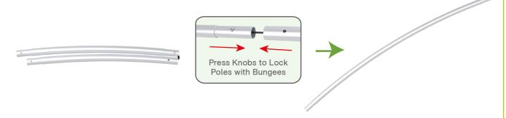
STEP 02 Connect long poles with corner poles according to labelings.
